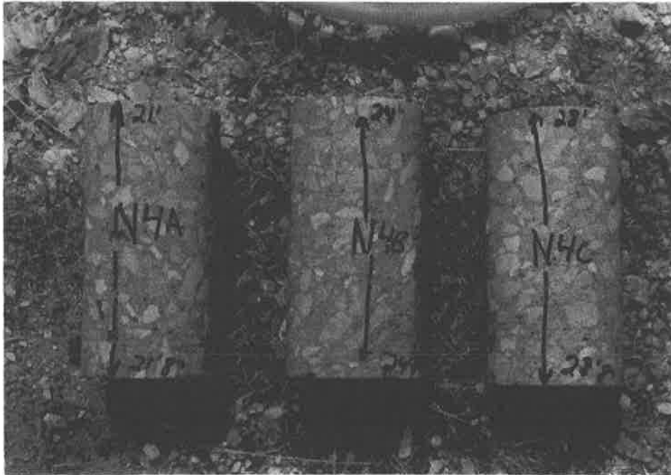
Photo 30 Core samples N4A, N4B and N4C from Lift #3 of the North Caisson. Lift #3 was placed by the central drop method with the same mix and slump as the two lifts above. No segregation of aggregate is apparent.
