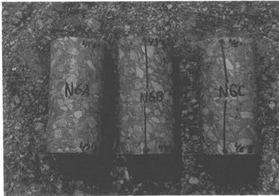
Photo 32 Core samples N6A, N6B and N6C taken from Lift #5 of the North Caisson. The lift was placed using Mix #1 by the central drop method. No segregation of aggregate was noted.
