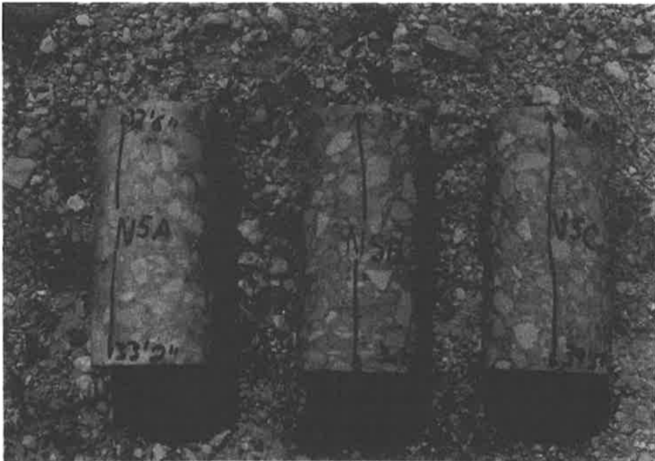
Photo 31 Cores N5A, N5B, and N5C were taken from Lift #4 of the North Caisson. Lift #4 was placed by tremie using Mix #1 with superplasticizer added. No aggregate segregation within the cores is apparent.
