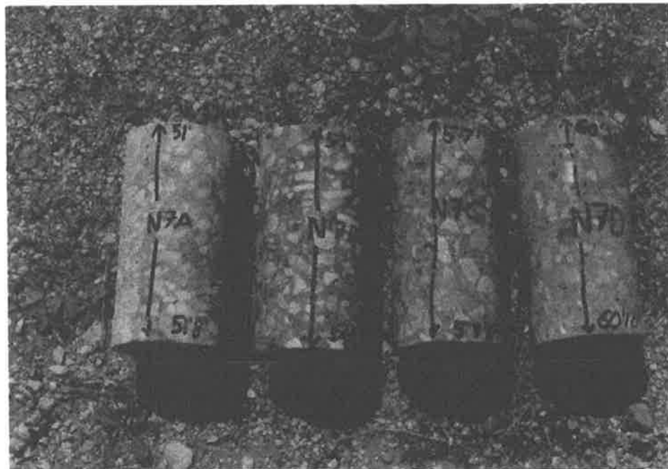
Photo 33 Core samples N7A, N7B, N7C and N7D from Lift #6 of the North Caisson. This lift was placed by the sloppy drop procedure with Mix #1. Some dark gray clay-filled voids can be seen in core N7D, however, no segregation of aggregate in the lift is apparent.
