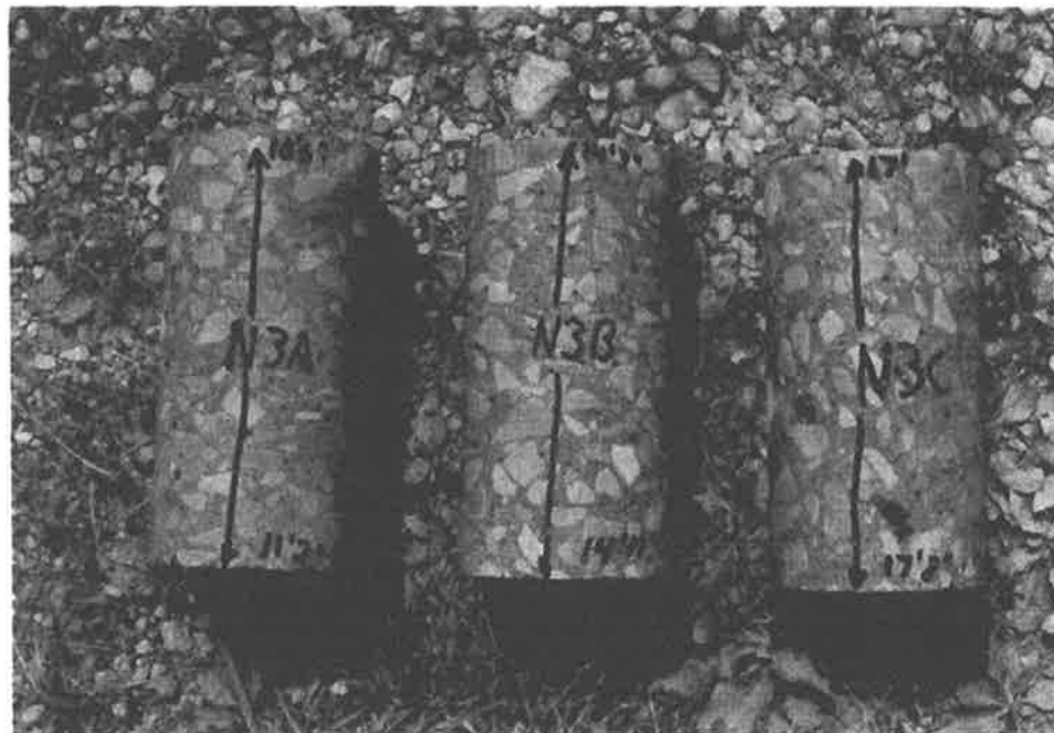
Photo 29 Core samples N3A, N3B, and N3C from Lift #2 of the North Caisson. Lift #2 was placed by sloppy drop procedures using concrete from the same truck as the lift above. No segregation is evident.
