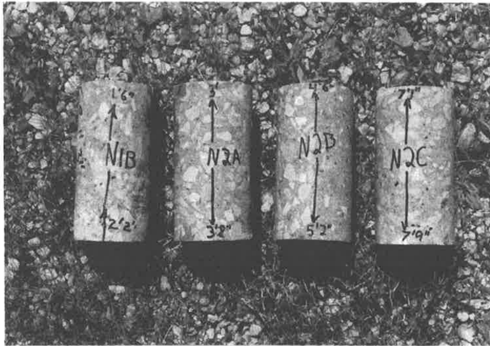
Photo 28 Core samples N1B, N2A, N2B and N2C from Lift #1 of the North Caisson. Note the vertical segregation of aggregate within core N2B. The concrete for these cores was placed by tremie using Mix #2. Core N1B was vibrated, while those below were not.
